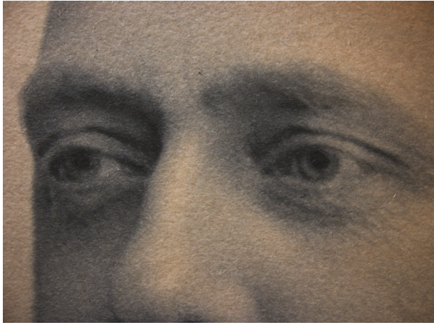
Figure 8a Detail of a platinotype photograph (6.3x magnification), showing clearly visible surface fibers.
