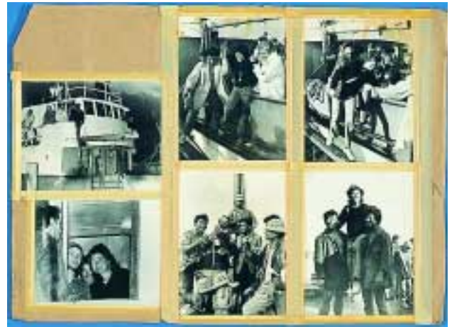
These photographs were attached to a scrapbook page using masking tape. The adhesive became sticky and stained the photographs.
