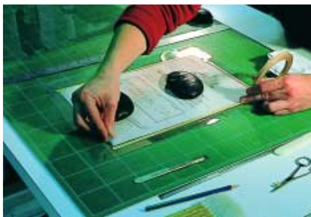
Double-sided tape being applied to the edges of a polyester sheet, during encapsulation of a paper item.
